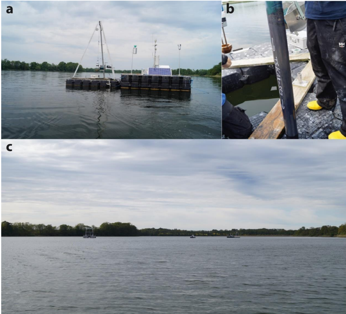
Figure 1.7: Images from Lake Tiefer See. (a) Weather monitoring set-up, (b) a freshly retrieved short sediment core, and (c) a platform for long core collection (left) and weather monitoring station (right).
