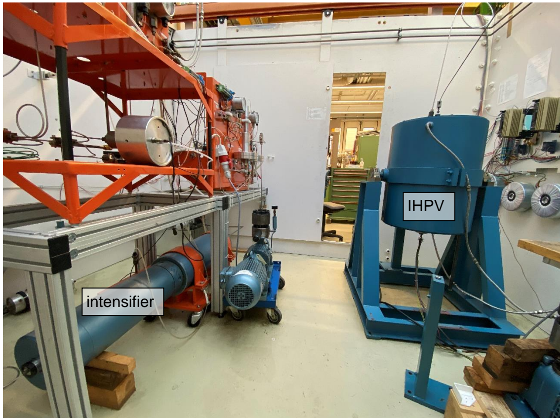
Figure 9: Internally heated pressure vessel of the GeoForschungZentrum (Potsdam). On the right side of the picture the vessel is shown in vertical working position, while on the left side, the whole pressure control system is visible, with the intensifier at the bottom.
