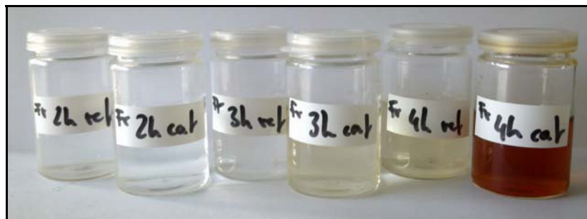
Figures A14: Comparison of HC products from fructose with and without the addition of borax after different reaction times. Shown are results from 20 ml glucose solutions (30 %) with (cat.) and without (ref.) the addition of 500 mg of borax for 1, 2, 3 and 4 hours at 140 °C.
