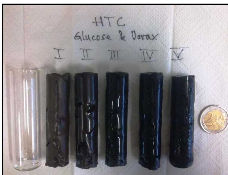
Figure A15: Image of representative Carbogels achieved from different amounts of borax added to a standard HTC recipe. Borax content: I) 100 mg, II) 250 mg, III) 500 mg, IV) 750 mg, V) 1000 mg. To show the gelation through the whole volume the glass vial i.e. reaction vessel is shown. A 2 Euro coin is added as size scale.
