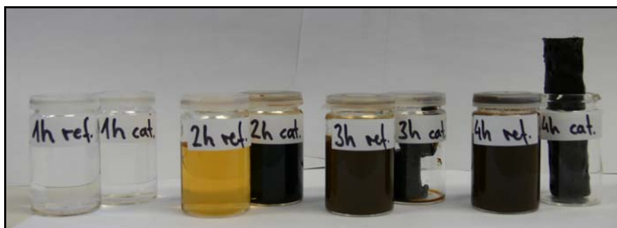
Figures A12: Comparison of HC products from glucose with and without the addition of borax after different reaction times. Shown are results from 20 ml glucose solutions (30 %) with (cat.) and without (ref.) the addition of 500 mg of borax for 1, 2, 3 and 4 hours at 200 °C.
