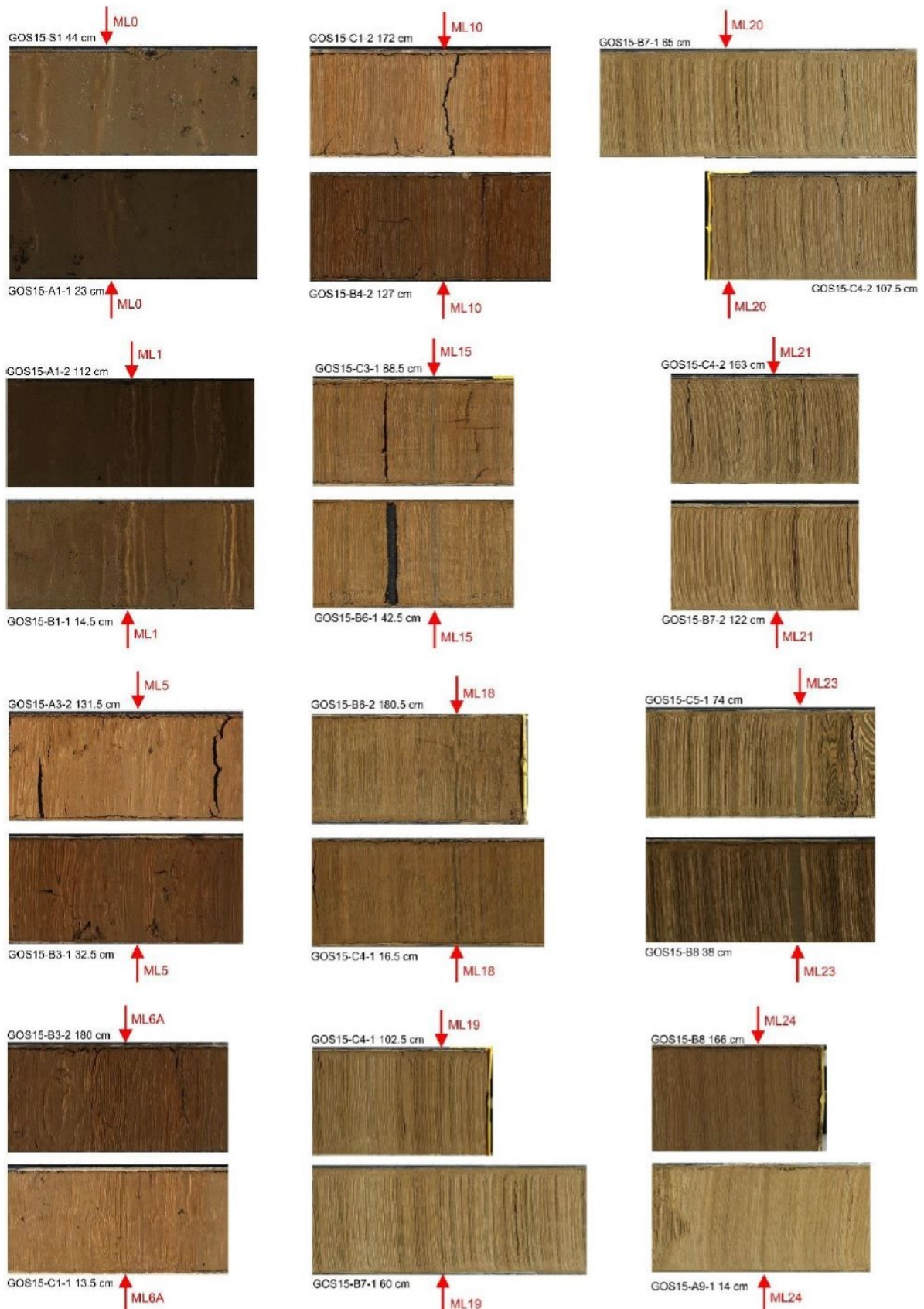
Figure S2-8: Examples of section correlation using marker layers.
