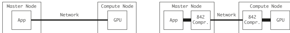
Figure 4.5: Compared to uncompressed data transfers (left), on-the-fly data compression may increase the effective bandwidth (right).
