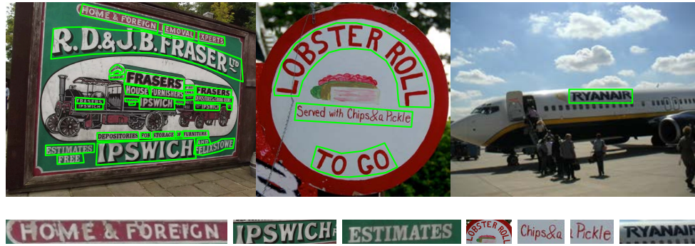
Figure 3.3: Depiction of examples of scene text found in real-world images. (Top) Three examples of full images containing scene text. Such images are used as input to a scene text detection network. The example images contain a wide variety of scene text. The image on the right contains an example of axis-aligned scene text. The image in the middle contains an example of curved scene text that is annotated using a polygon. The image on the left side contains a wide variety of challenging scene text examples. (Bottom) Examples of cropped word images that are used as input for the task of scene text recognition.
