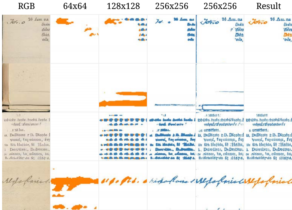
Figure 4.18: Classified clusters produced by intermediate layers. The clusters were produced by applying k-Means on the activations of the synthesis network of a trained StyleGAN model (see figure 4.17). The numbers on the top indicate the spatial size of the intermediate feature maps of the synthesis network in pixels. The left-most column shows the RGB images generated by the trained StyleGAN model. Blue color highlights pixels classified as printed text, orange pixels represent the handwritten text class, and white pixels depict background pixels. The clusters appear to be noisy. However, by applying a well-designed algorithm to the given feature maps, we can reduce the number of false labels by a large margin. The resulting segmentation images are shown in the right-most column.
