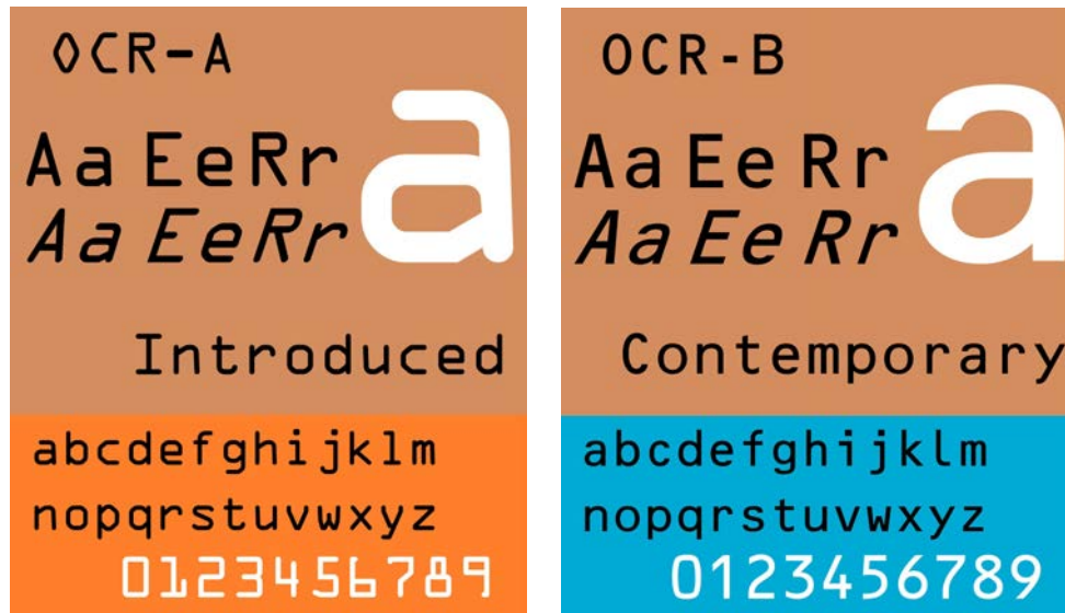
Figure 2.1: Standardized font faces for early OCR of printed text. (left) OCR-A, 2 (right) OCR-B 2
