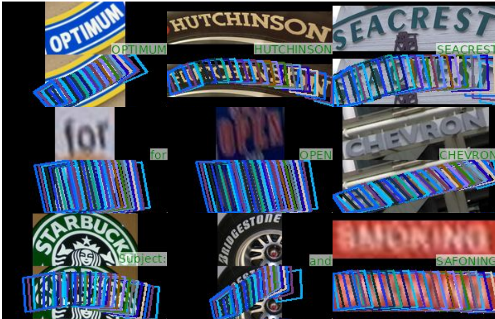
Figure 3.18: The qualitative evaluation of our proposed scene text recognition approach shows that our model learned to follow the slope of words, even if they are curved. The top two rows show some correct results of our proposed model. The last row shows three typical failure cases of our model. We are certain that these failure cases can be alleviated by using more training samples with curved and severely degraded text instances.
