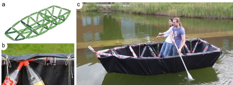
Figure 9: A functional boat is assembled following the embossed hub IDs. (b) The bottle frame is simply covered by a tarp. (c) The fabricated boat seats two.
