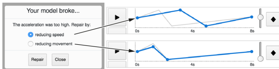
Figure 42: If the user-defined animation breaks the model, TrussFormer offers to automatically reduce the speed or the motion range.
