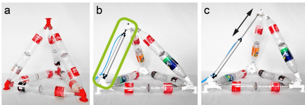
Figure 27: (a) The static tetrahedron (b-c) is converted into a deformable structure by swapping one edge with a linear actuator. The only required change is to introduce connectors that enable rotation.
