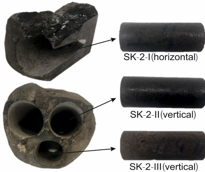
Figure 4.1 Samples SK-2-I-III taken from one core piece recovered from borehole SK-2 in 355 m depth. The dimensions of the samples were 61.3 mm length and 24.9 mm in diameter.
