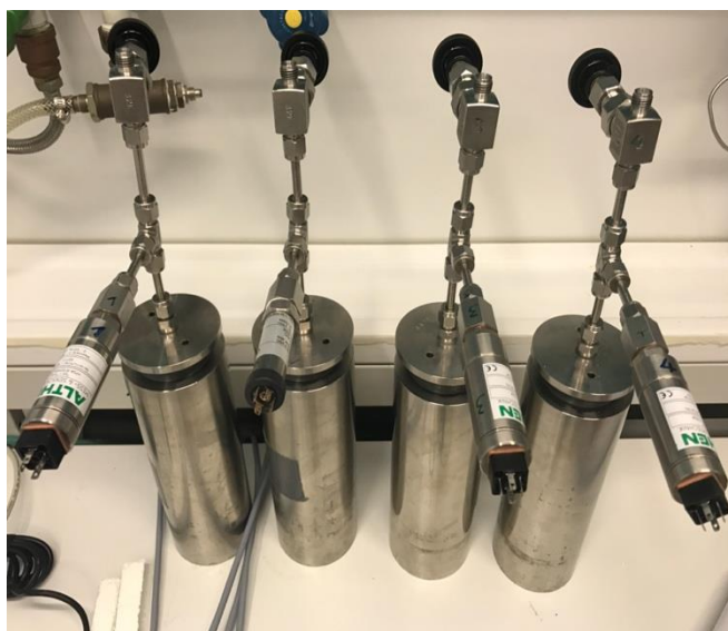
Figure 2.11 Picture of the stainless-steel pressure vessels. Each of them has a volume of 420 ml.
