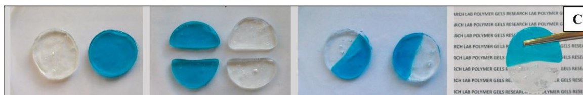
Figure 1.7: Hydrogels of copolymers of stearyl methacrylate and acrylamide at concentration of 5 wt. % in 0.5 M NaCl solution. One of the gel samples is colored with methylene blue for clarity. After cutting into the gels in two pieces and pressing the fractured surfaces together, they merge into once single piece. 109
