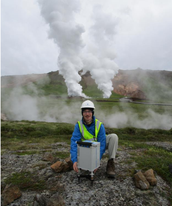
Figure 6. Time-lapse measurements with the Scintrex CG5 relative gravity meter at the Þeistareykir geothermal field.
