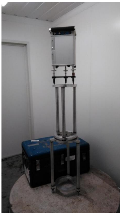
Figure B4. Measuring setup at Þeistareykir for determination of the free-air vertical gravity gradient with the help of a CG5 Scintrex gravity meter and a tripod; gravity measurements were performed directly on the concrete pillar, at 60 cm and at 120 cm above the pillar.
