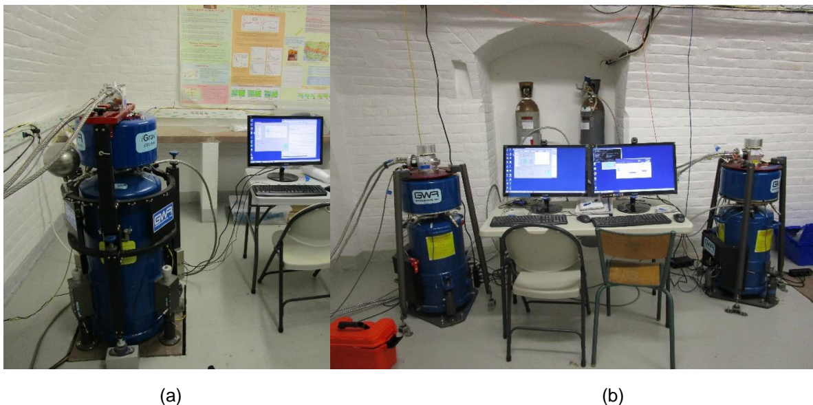
Figure A2. Measuring setup for iOSG023 (a) and iGravs 032 and 015 (b) at the gravimetric observatory J9 in June 2017; with each instrument connected to a separate helium cooling system and data acquisition unit.
