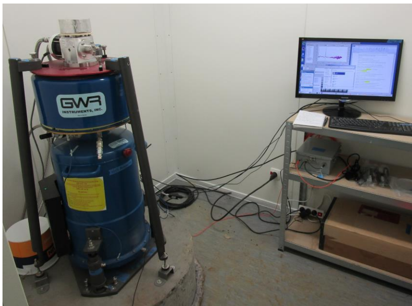
Figure 8. Continuous gravity observations with the iGrav superconducting gravity meter (SG) installed on a decoupled concrete pillar in the back room of the gravity stations at Þeistareykir; setup shown for iGrav015 at the reference station.
