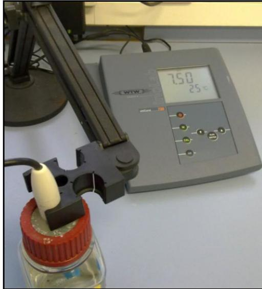
Figure 9: WTW inoLab pH/Cond 720 for determining the pH-value
