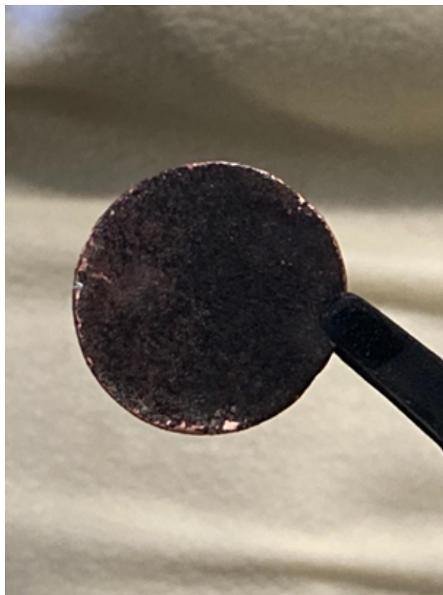
Figure A.13.: Photograph of an electrode of Kynol CC after 100 cycles. No metallic sodium can be seen, neither in the electrode, nor in the separator (not shown).
