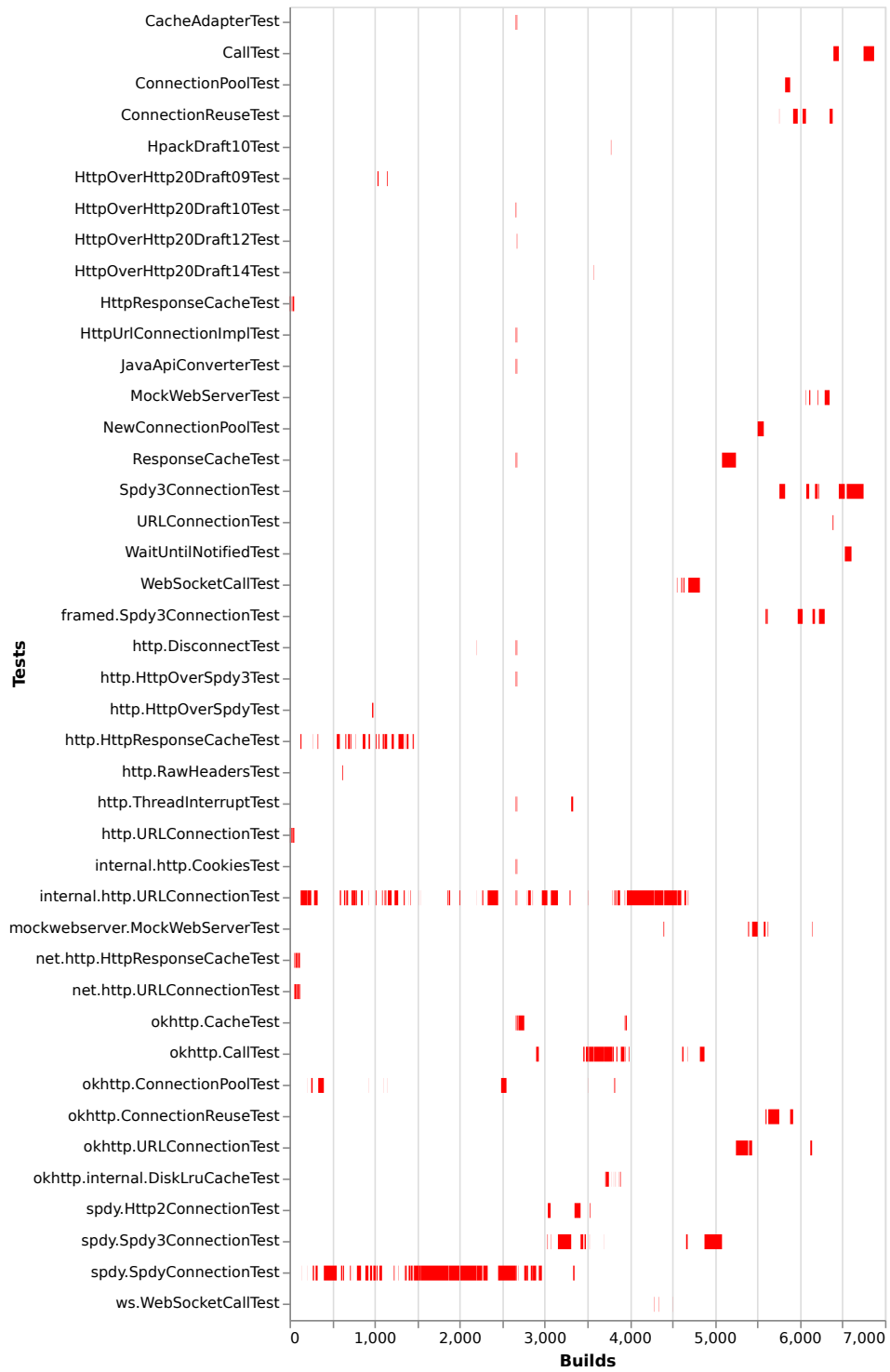
Figure 5.5.: Failure histories for the okhttp project. Each red bar indicates a test failure for a given build number.
