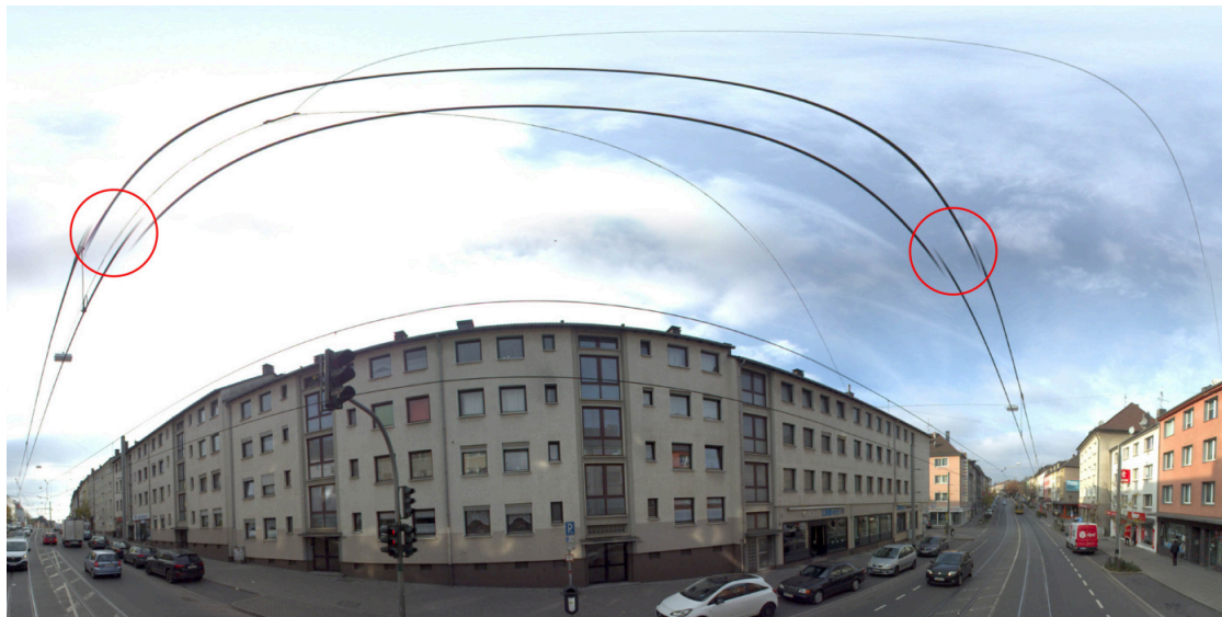
Figure 6.7: Visualization of a panoramic image from the Essen dataset. Image stitching artifacts are visible at the catenary cables (red circles).
