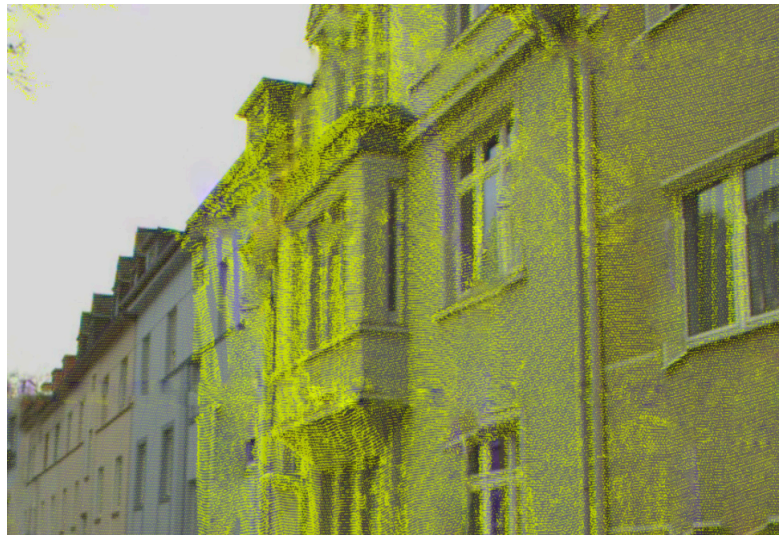
Figure 6.6: Visualization of a panoramic image with the points of a 3D point cloud from the Essen dataset projected on top of it.
