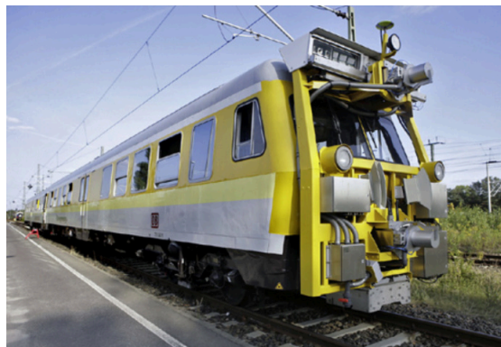
Figure 3.9: Measurement train “Limez III”. LiDAR scanners are attached to the front of the train. Figure from Wirth (2008).
