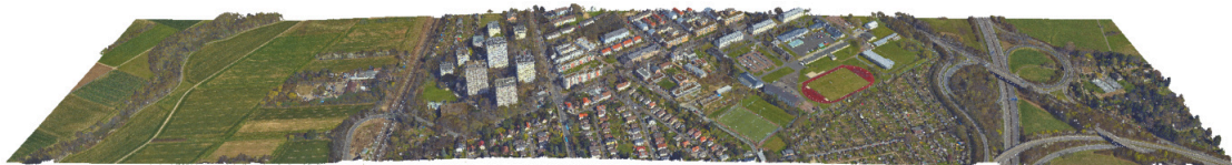
Figure 1.1: Visualization of an airborne 3D point cloud depicting from left to right: Meadows around a river, agricultural land, train tracks, residential area, sports areas, allotment gardens, a highway, and forest area.
