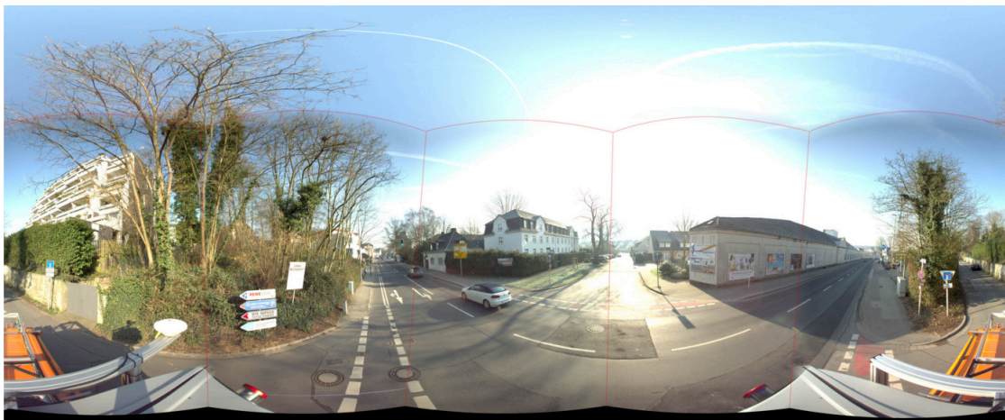
Figure 6.1: Visualization of a panoramic image from the Essen dataset taken by five cameras oriented sideways and one oriented upwards. The regions of the individual images are approximately bordered in red. The measuring car is partly visible.
