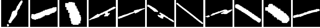
Figure 3.8: Examples of rendered 132 by 132 pixel images of detected road marking clusters. White pixels represent areas where a road marking was detected, black pixels represent background.
