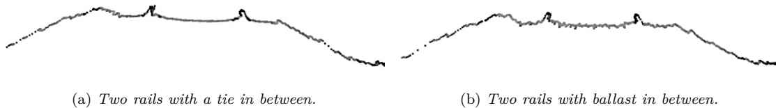
Figure 3.12: Two scan profiles of a railroad track on a ballast hill. Grayscale colors represent the intensity values of the points.
