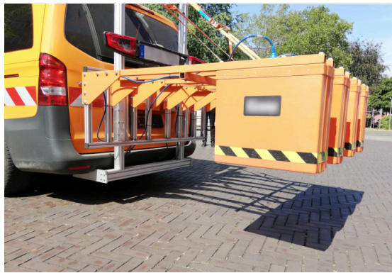
(a) Four GPR antennas mounted on the back of a car. (b) GPR hand cart. Figure from Geophysical Survey Systems (2018).
