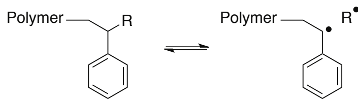
Scheme 1: Basic principle of Controlled Radical Polymerizations: Reversible interchange between dormant and active chain ends.
