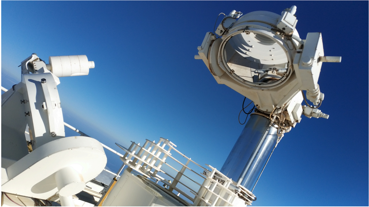
Figure 2.3: The coelostat mirrors of the the Vacuum Tower Telescope (VTT) at a height of 38 m in September 2018.
