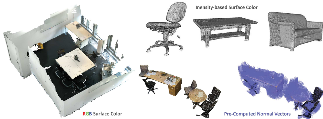
Figure 2.5: Typical representations of indoor point clouds include Red-Green-Blue (RGB) or intensity-based point clouds, which may include additional attributes e.g., pre-computed normal vectors.
