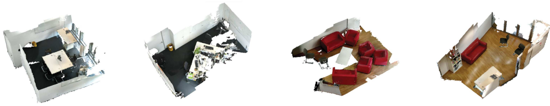
Figure 4.1: Examples of indoor point clouds captured using a commodity mobile device. These scans contain between 200 000 to 500 000 points, and feature RGB color values in addition to spatial attributes.
