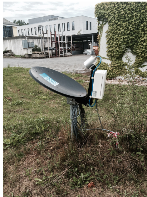
Figure 3: Micro Rain Radar of the University of Potsdam in Golm. From Breier (2015).
