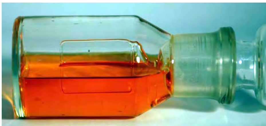
Figure 2.13: Photo of the device used for the measurement of the lamella lifetime.
