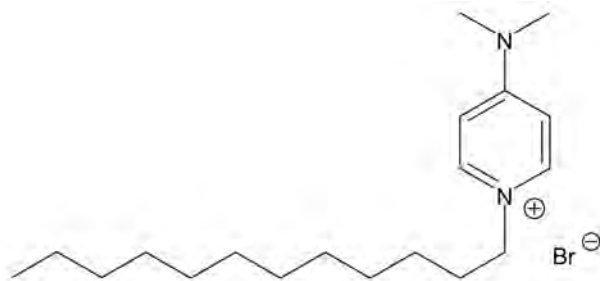
Figure 2.1: Chemical structures of the cationic amphiphile 1-dodecyl-4-dimethylaminopyridinium bromide, C12-DMPB
