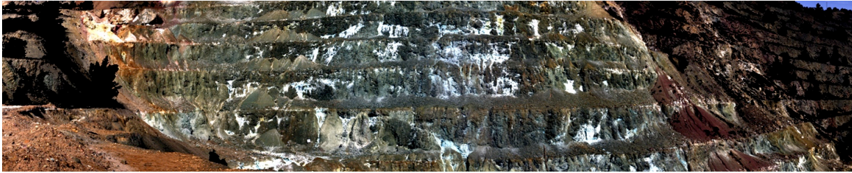
Figure 38 NDVI & shadow masked reflectance field scan. Vegetation and areas of shadow (high SNR) are masked out and shown in black. (RGB composition: R: band 63, G: band 38, B: band 13.)
