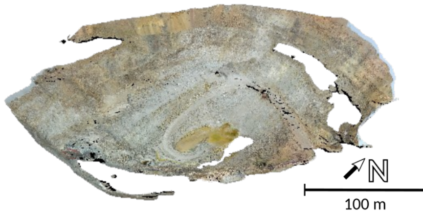
Figure 44 The resulting 3D model, textured with the orthophoto mosaic of all available Nikon photos.
