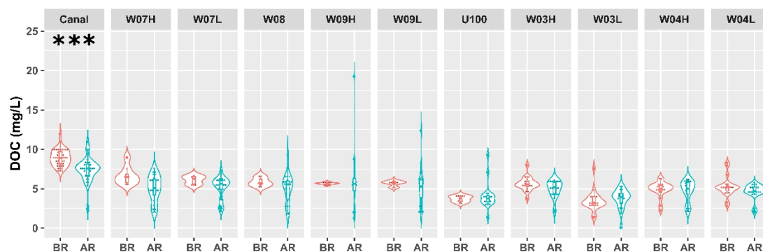
Fig. 3.16 Violin plots of the variation of dissolved organic carbon (DOC, mg/L) in the river and observation wells. ‘*’ was used to denote the significance level (***)represents P < 0.0001 ). Boxplots are included within the violin plot. The “BR” denotes to before reconstruction (from 2007 July to June 2013); “AR” denotes to after reconstruction (from June 2013 to February 2).
