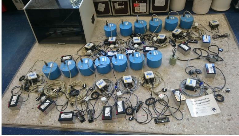
Figure 2.7: All seismometers were aligned during the lab-based huddle test, before the deployment in the field. Data-Cube digitizers and sensors were powered by batteries.
