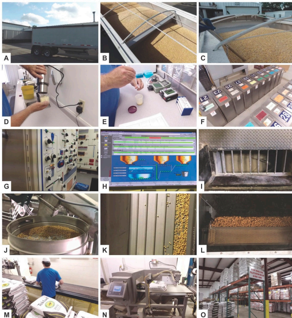
Figure 2. Overview of some work steps in the production of an extrusion diet in large scale. (A,B) The first step in production of mouse diets is the selection, procurement and approval of high quality bulk ingredients. In this regard, each company might have a different source of raw materials. (C–E) From each bulk, samples are taken and screened by a well-trained technician for mycotoxins (e.g., aflatoxin, vomitoxin, fumonisin), protein, fat, fiber, and moisture using near infrared spectroscopy and approved/certified test kits. (F) When quality is assured, each lot of raw material receives a lot number that is used to track each ingredient through the entire production process. (G–I) The different ingredients are mixed together in a certified mixer, in which flow from ingredient bins, scales and processing is critically monitored. (J–L) To produce an extruded diet form, the mixed ingredients are sent first to a post grind hammer mill and then to an extruder, in which the mixture is forced through a die. In this device, the product is expanded by a stream that is injected under pressure. In a next step, the product is passed through a dryer and several screeners to ensure that no metallic traces or other unwanted compounds are passed through. The moisture and bulk density of the product is evaluated and recorded. (M,N) Finally, the diet is packed in packing lines and once validated for unwanted stray metal particles by an in-line metal detection capability. (O) All diets are stocked in suitable facilities from which they are quickly retrievable on demand. All images were kindly provided by Dr. Jörg Lesting (Envigo Teklad Diets, Madison, WI, USA). A well-arranged movie showing the complete manufacturing process is viewable online at: https://www.envigo.com/p/teklad/ .
