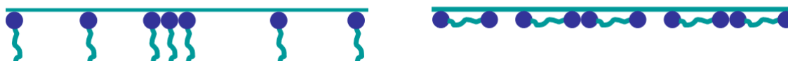
Figure 4-1: Methods to locate organic groups to the surface of the pores in mesoporous silica. Grafting on the left and painting on the right.
