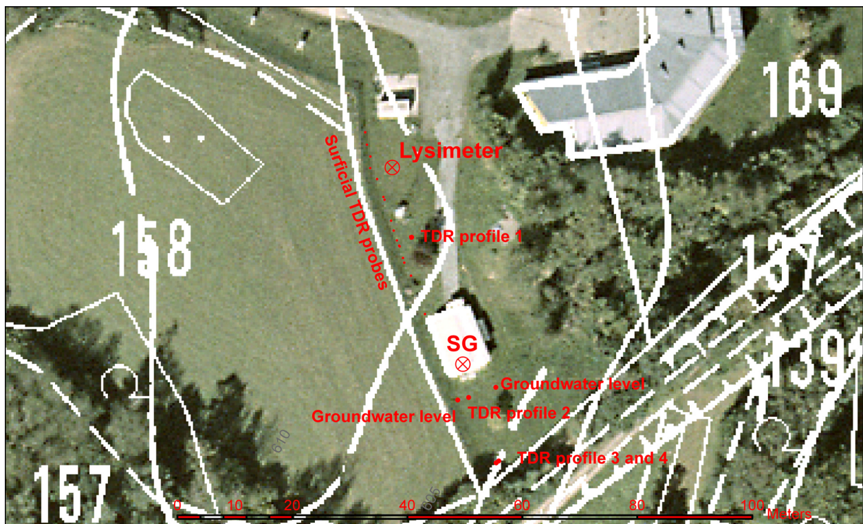
Figure 4.1: Lysimeter, SG and different hydrological sensors in combination with an ortho-image of the study site (white lines: contour map and land register map).
