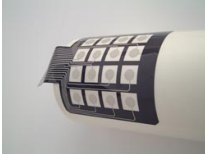
Figure 3.7(b): Keypad elements can be installed also on curved surfaces [www.screenotec.com] .
