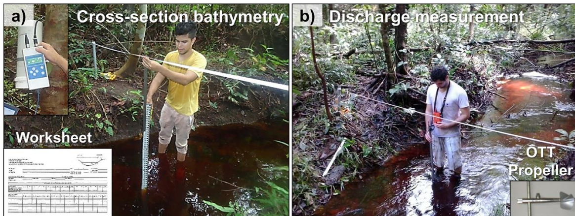
Figure 31 – Measurements of (a) bathymetry and (b) discharge in stream gauges of GEB for runoff estimation. Source: (Barbosa, 2015).
