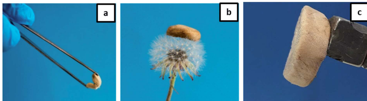
Fig. 6 Photographs demonstrating the properties of an aerogel: (a) flexibility; (b) ultra-light weight; (c) movement by external magnet.
