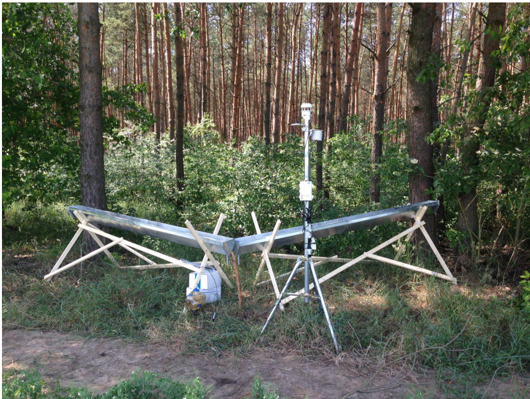
Figure 8.6 Setting of weather stations in the forest (zero line, -35 m and -70 m) with rain gauges.
