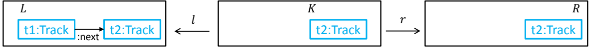
(a) Example graph rule b = \langle (L \leftarrow K \rightarrow R), \text{true}, \text{true} \rangle
