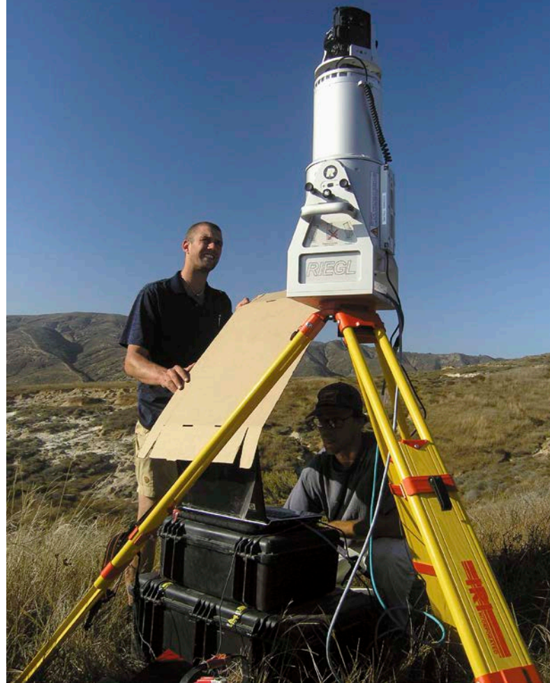
Photo taken with a Lidar to get a surface model of the area of Santa Cruz Island (Southern California), down to the centimeter.
