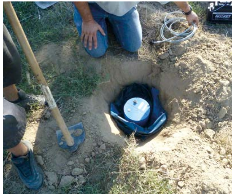
Katrin Hannemann and Agostiny M. Lontsi, PhD students at the University of Potsdam, are checking signals of a seismometer in Greece; these data are also used by Annabel Händel.
