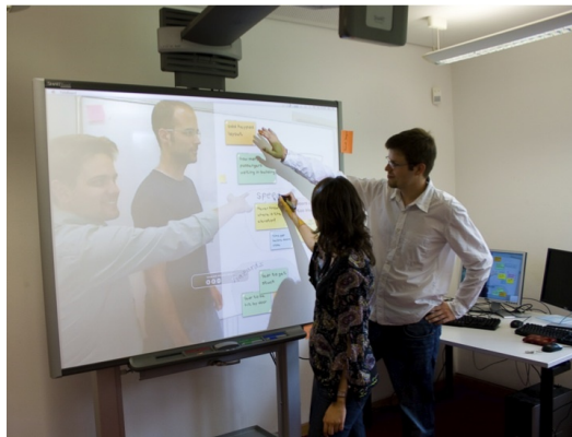
Figure 3.1: Tele-Board user scenario (copied from Gumienny, Gericke, Quasthoff, Willems and Meinel (2011)). A team distributed across different geographic locations is working on a shared digital whiteboard interface in real-time. The team in one location can see the team in the other location via a video conferencing overlay.
