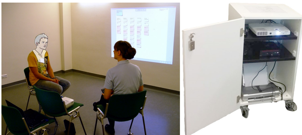
Figure 5.12: Tele-Board MED setup at a hospital ward. In the initial setup (left), a laptop and projector were installed in the treatment room positioned on chairs. In order to improve the mobility, a trolley was built to store and quickly move the devices (right).
