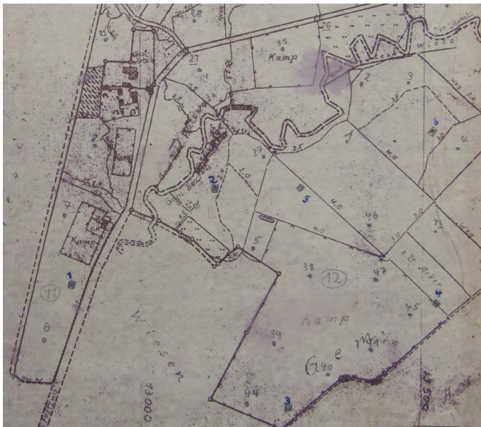
a) Section of a forestry map at scale 1:10,000, in which the positions of site investigation pits are marked with a small square and the corresponding pit number.
