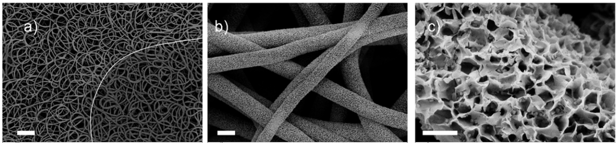
Figure 3.22. Crystallized micron-sized PCL fiber mats were nicely coated (b,c), however the increase in plasma treatment time revealed no dramatic increase in coating area (dark zone indicated in a) (135 min crystallization time, 30min pre-soaked, 2x10min plasma, air, 18W; scale bars: a) 100 \mu\text{m} , b) 10 \mu\text{m} , c) 2 \mu\text{m} ).
