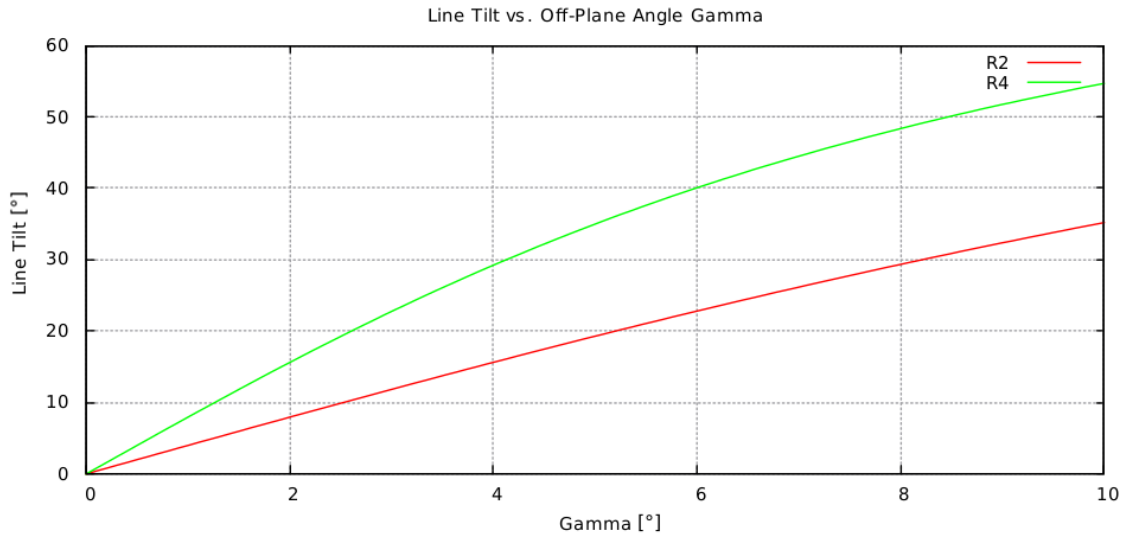
Figure A.23.: Line tilt introduced by off-plane angle \gamma . Red is for an R2 grating ( \theta = 63.4\hat{\text{A}}^\circ ) and green for R4 ( \theta = 76\hat{\text{A}}^\circ ).
