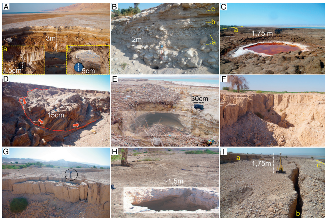
Fig. 10. Geology, structures and sinkhole morphologies at Ghor Al-Haditha. A: Mud-flat deposits, comprising laminated silt and clay, locally interbedded with evaporite layers up to 1.5 m thick (a) and idiomorphic halite crystals (b). B: Alluvial fan deposits, comprising poorly consolidated gravels (a), coarse to fine grained sand (b), with clayey topsoil (c). C: Typical shallow and wide sinkhole (depth to diameter ratio D \approx 1.5 \text{ m}/17 \text{ m} = 0.09 ) with gentle slopes in the mud-flat deposits about 100 m north of the alluvium/mud-flat contact (a). Note tripod for scale. D: Listric normal fault bounding outward-rotated blocks of a landslide or slump into a dry stream channel in the rheologically weak mud-flat deposits. A tunnel has been carved into the strong salt layer whose overhanging side points towards the Dead Sea. E: Small overhanging sinkhole in a mud-salt sequence locally dominated by thin but strong evaporite layers. Highlighted by contrast stretching is the wet mud filling. F: Typical deep sinkhole with high D = 12 \text{ m}/23 \text{ m} = 0.52 in the rheologically strong alluvium. G: Inward-tilted and overhanging faulted blocks at the margin of a sinkhole in the alluvium. Note person (circled) for scale. H: Overhanging side walls of sinkhole in the alluvium, here highlighted by contrast stretching. I: Up to 2 m high normal fault scarp (a) and ca. 4 m deep cracks (b) in the alluvium about 20 m from the alluvium/mud-flat transition (c).
