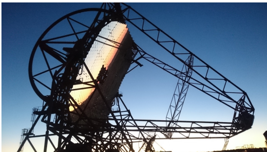
Figure 3.3: The fifth telescope, which was added in 2012, in twilight (September 2017). On the left hand side, the mirror facets, which form the dish. Situated at the end of the leverage on the right is the camera.
