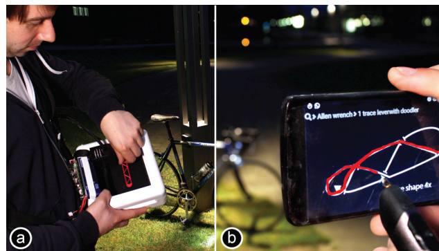
Figure 1: According to our survey, one use case of mobile fabrication is to fix things that break while on the go. This user, for example, fabricates a hex key to fix his broken bike light using either (a) a custom “mobile” 3D printer or (b) a “human-assisted” 3D printer based on an extruder pen. We drive both using a mobile phone running our custom app.
