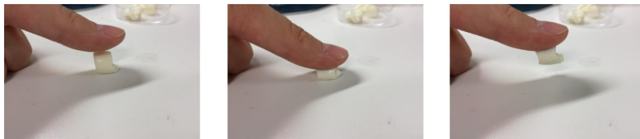
Figure A42. Gentle compression on 2 wt.% g-CN-AHPA hydrogel and its adhesion to finger.
