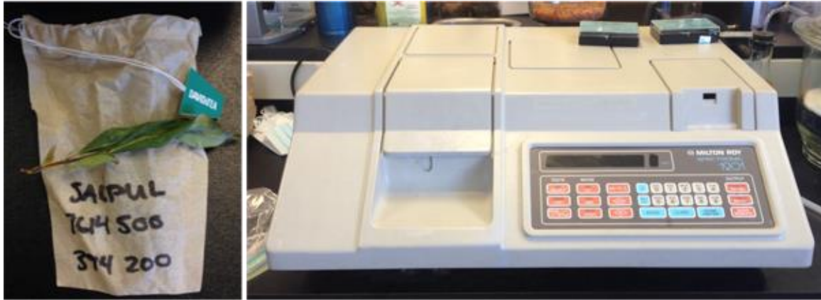
Figure 1-5 Left: Example of a silica gel-preserved biomass sample ( Salix pulchra ) prior to grinding and extraction. Right: Spectronix 1201 spectrophotometer used to measure absorbance ( A ) and pigment concentrations.
