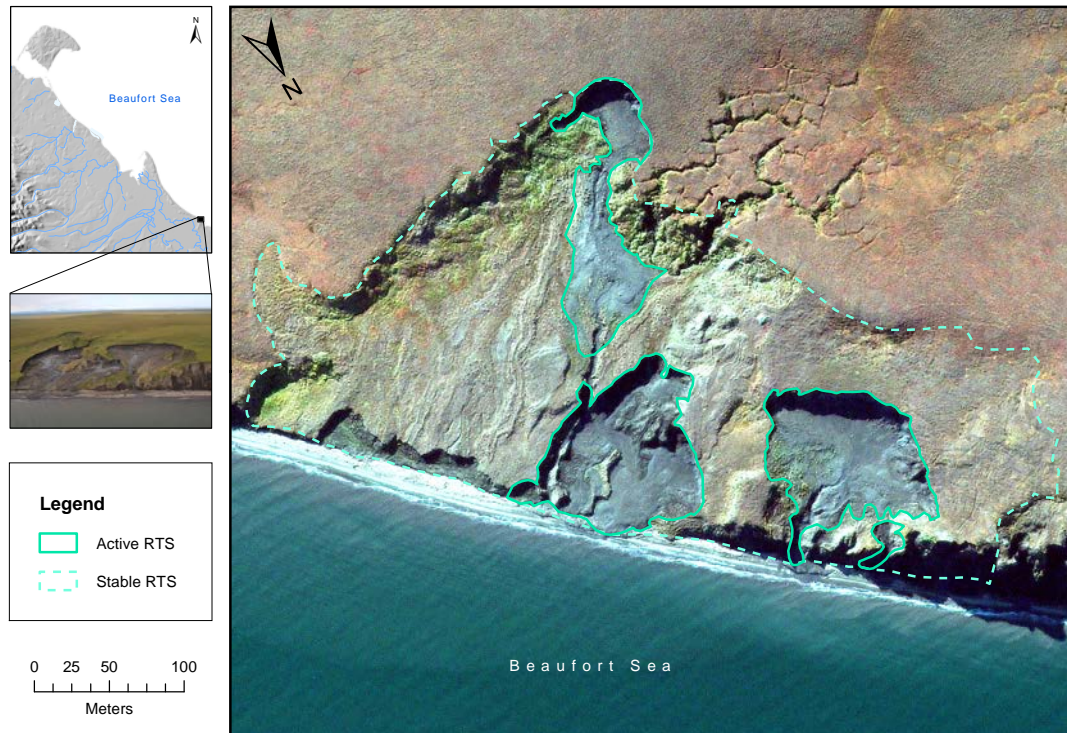
Figure 3.2 – GeoEye image from July 18 th 2011 illustrating the differences between active and stable Retrogressive Thaw Slump (RTS)s. The depicted RTS is located in the eastern part of the study area, at King Point (segment 32). The oblique photograph was taken from a helicopter during fieldwork in July 2015.
