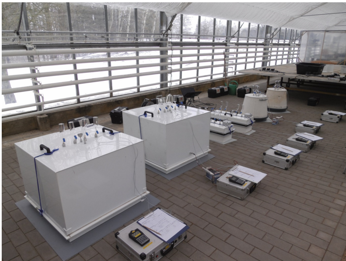
Fig. 2.1 Experimental setup at the Institute for Landscape Biogeochemistry of the Leibniz Centre for Agricultural Landscape Research (ZALF), Müncheberg, Germany. The picture shows simultaneous measurement in flow-through (continuous sampling) and non-flow-through (discrete sampling) mode for all six tested chambers. The right chamber of each design represents the non-vented chamber (without fan and pressure vent)
