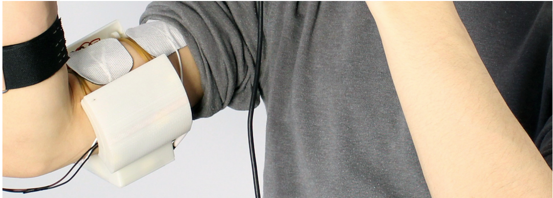
Figure 15: Detail of the electrical muscle stimulation component. Here, it stimulates the user’s biceps brachii muscles causing an involuntary contraction that resembles force feedback.
