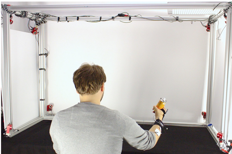
Figure 98: This affordance++ prototype uses an Optitrack setup for tracking.
