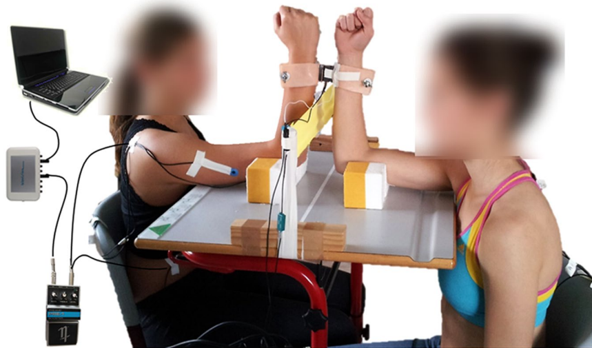
Figure 1. Setting of interacting subjects. Interaction of two subjects during measurement of the abdominal external oblique and triceps brachii muscles and the triceps tendon by piezoelectric MMG-sensors. The signals are conducted across an amplifier to an A/D-converter and are recorded by the software NI DIAdem 10.2 on the measurement notebook (see in 26 ).
