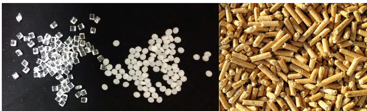
Figure 2. Polystyrene (PS, left) and polyethylene (PE, middle) particles used for the exposure experiments. Wood pellets (right) were used as a natural reference surface.
