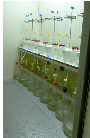
Figure 6. The setup of the chemostat system in a climatic chamber for study II.
