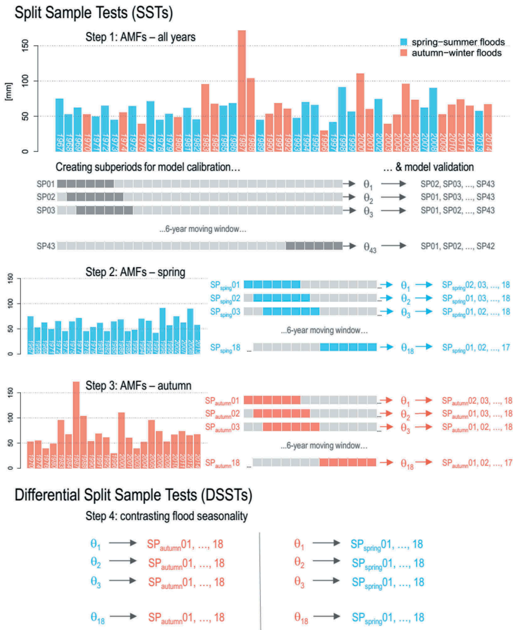
Figure 2. Illustration of the methodology used for testing the transferability of calibrated hydrological model parameters based on the principles of the split-sample test (Step 1) and the differential split-sample test (Step 2) (Klemeš 1986). The generalization of those schemes, i.e. the 6-year moving window, is adapted from Coron et al. (2012). The numbers in this illustration stem from the study catchment Kråkfoss. Note that a 5-year spin-up period is applied for each sub-period in both calibration and validation modes. Moreover, for Steps 2–4, the model is run over continuous time periods and only the relevant years are used for model evaluation.
