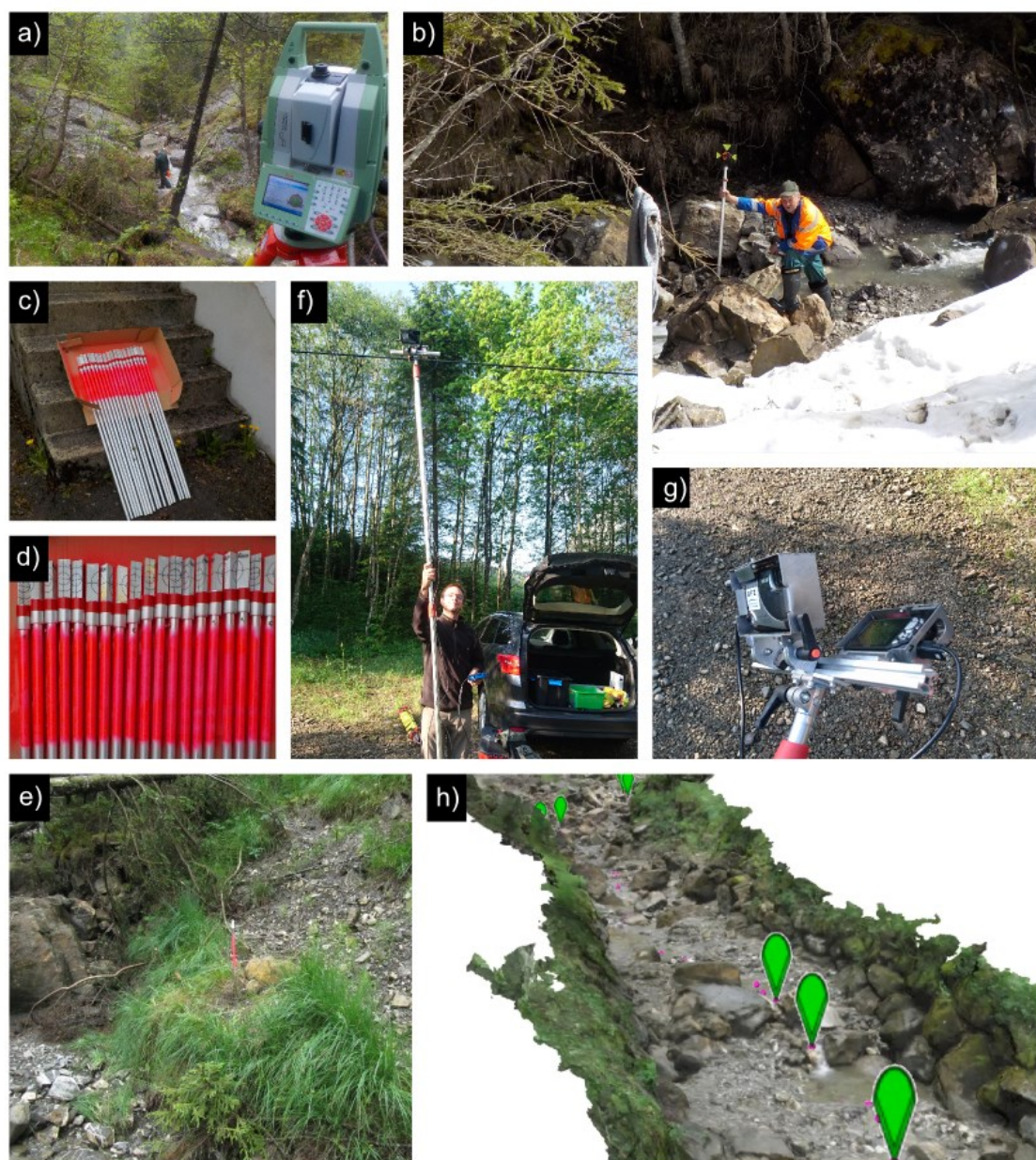
Fig. 59: a) the Leica total station during a typical survey of long profile, channel banks and fix point markers in the Erlenbach, b) assistant holds the reflector required for thalweg and bank survey point measurements, c),d) preparation of reference markers, e) reference markers deployed in the study reach, f) the 3 m long mount of the digital cameras used for the photogrammetric surveys, g) the camera mount on top, h) the final 3d model of the reach created based on the photogrammetric images created with Agisoft PhotoScan Pro.
