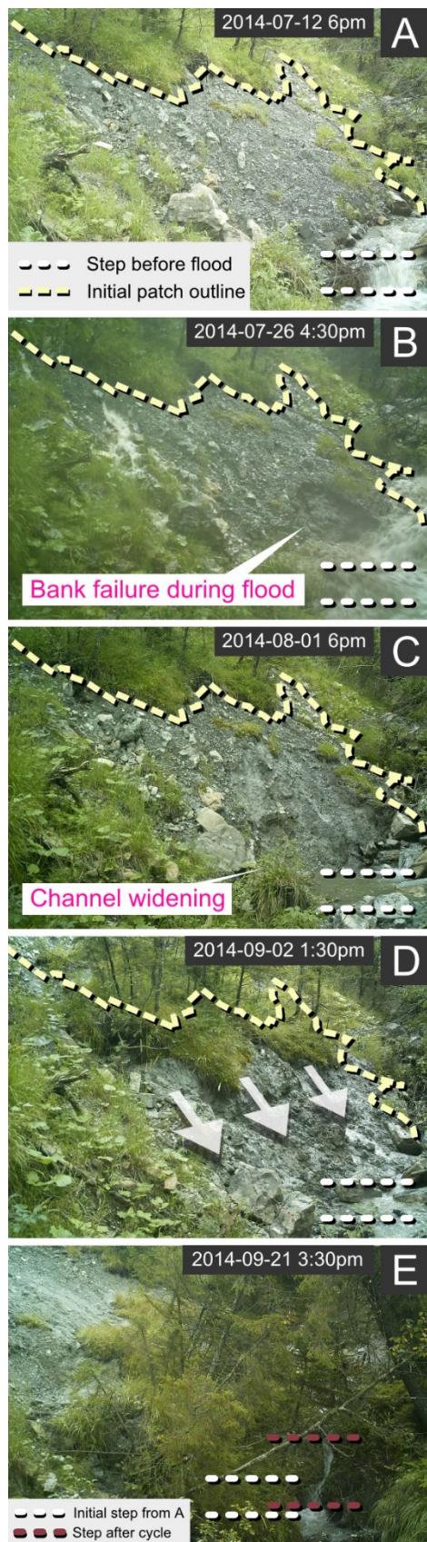
Fig. 17: The phases of the feedback cycle captured by the time-lapse camera. A: the Erlenbach stream with an alluvial step at the downstream end of a suspended landslide, B: flood causes step destruction and an immediate bank failure, C: channel width increases due to step destruction, D: landslide enters a phase of integral motion as a response, E: final blockage of the channel with hillslope material forming a new step (initial step position indicated in red) leading to landslide stabilization. Note: the camera pan between D and E was considered for the calculation of the displacement rates. Large image versions can be found in the Appendix C, as well as in the movie in Appendix B.
