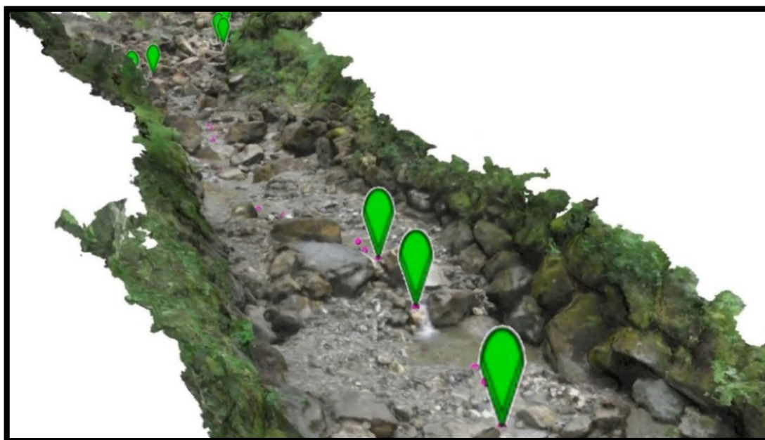
Fig. 13: An example of the three-dimensional model of the Erlenbach. The image shows the meshed dense point cloud rendered with the texture from the images in Agisoft Photoscan. The pink points on the channel bed indicate the total station measurements of the thalweg (water flow path during base-flow conditions). The green markers indicate the position of alluvial channel steps identified with the automated algorithm by Zimmermann et al., 2008. A link to a video of the model can be found in Appendix A.
