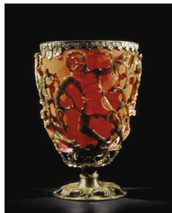
Figure 1.1.: The Lycurgus Cup, manufactured in the 4th century. Its red colour upon transmission and green colour upon reflection of light stem from nanoparticle colourants. [3]
