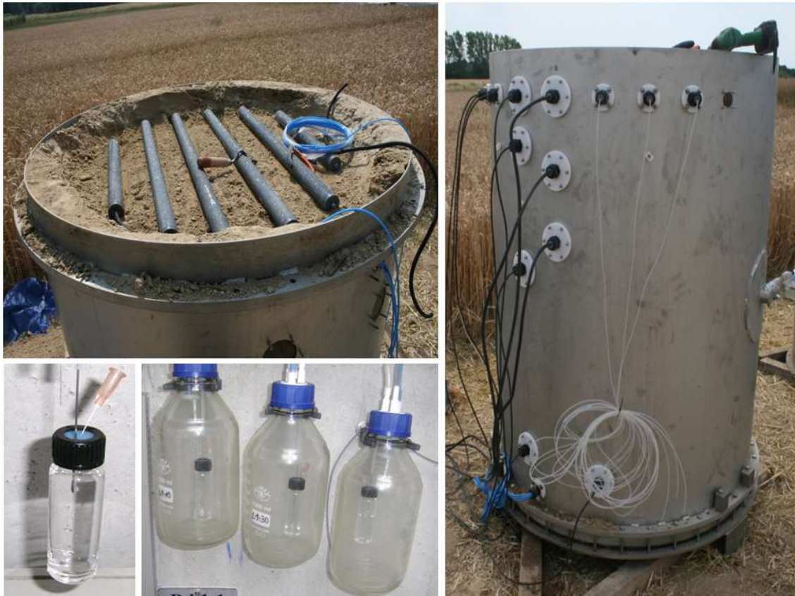
Figure 1.4: Weighing lysimeter (UMS, Munich, Germany) during sensors installation process (right); suction cup rake (SIC40, UMS, Munich, Germany) at the lysimeter bottom (1.45 m depth) consisting of six porous tubes (left above) and glass bottle attached to the lysimeter tank (left below). Photos: Institute of Soil Landscape Research, Leibniz Centre ZALF.
